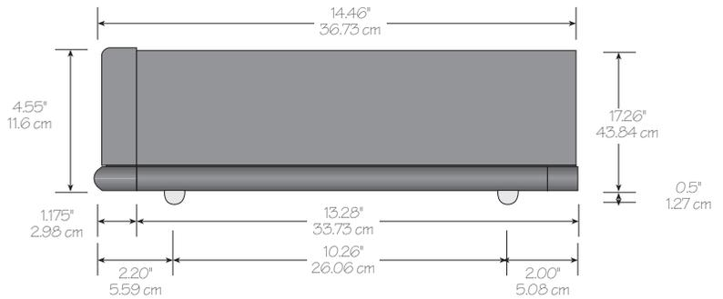
(note that additional space must be allowed for connections *behind* the unit)
